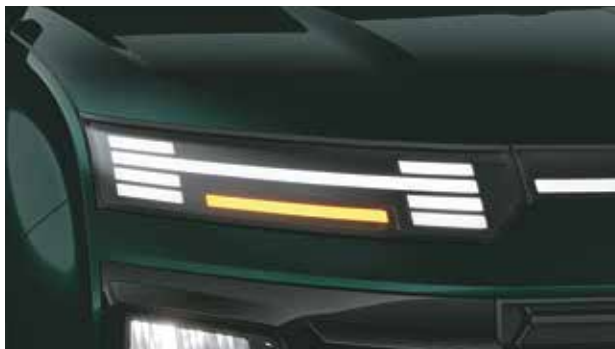
LED turn signal with sequential function
