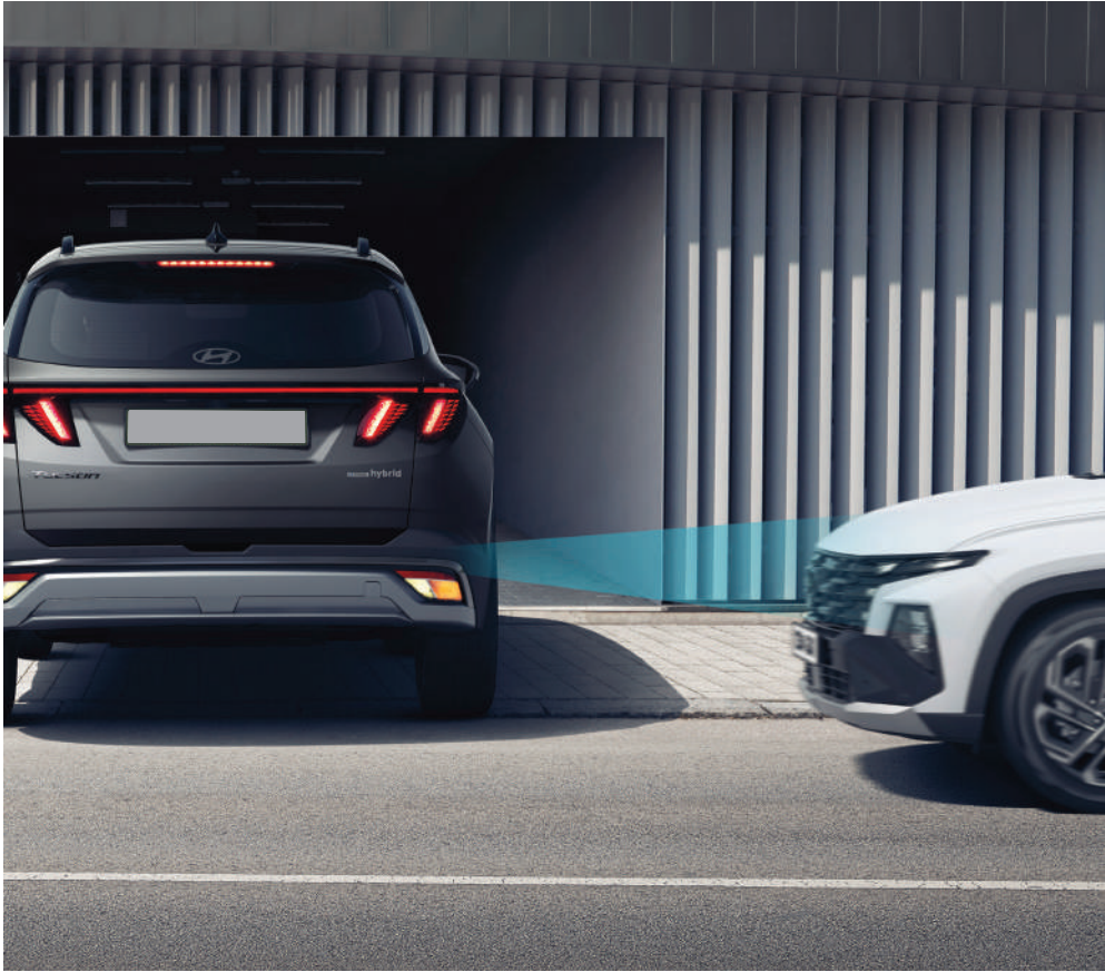
Parking Collision-Avoidance Assist (PCA) Reverse Parking Collision Avoidance Assist (PCA) provides a warning if there is a risk of collision with a rear object while reversing. After the warning, if the risk of collision increases, it automatically assists with emergency braking.
