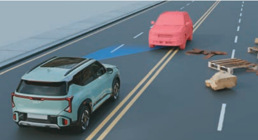
Front Collision-Avoidance Assist-Lane Change Oncoming (FCA-LO)
